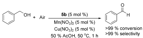
Scheme 4. Aerobic oxidation of benzyl alcohol using 5a or 5b with Mn II /Cu II co-catalysts (modified Minisci condition).
